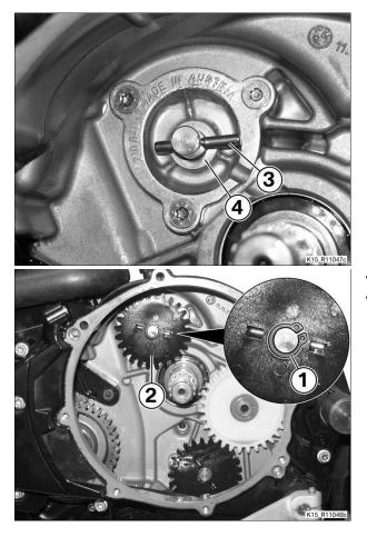
Install oil delivery pump gear (2).Install circlip (1).
